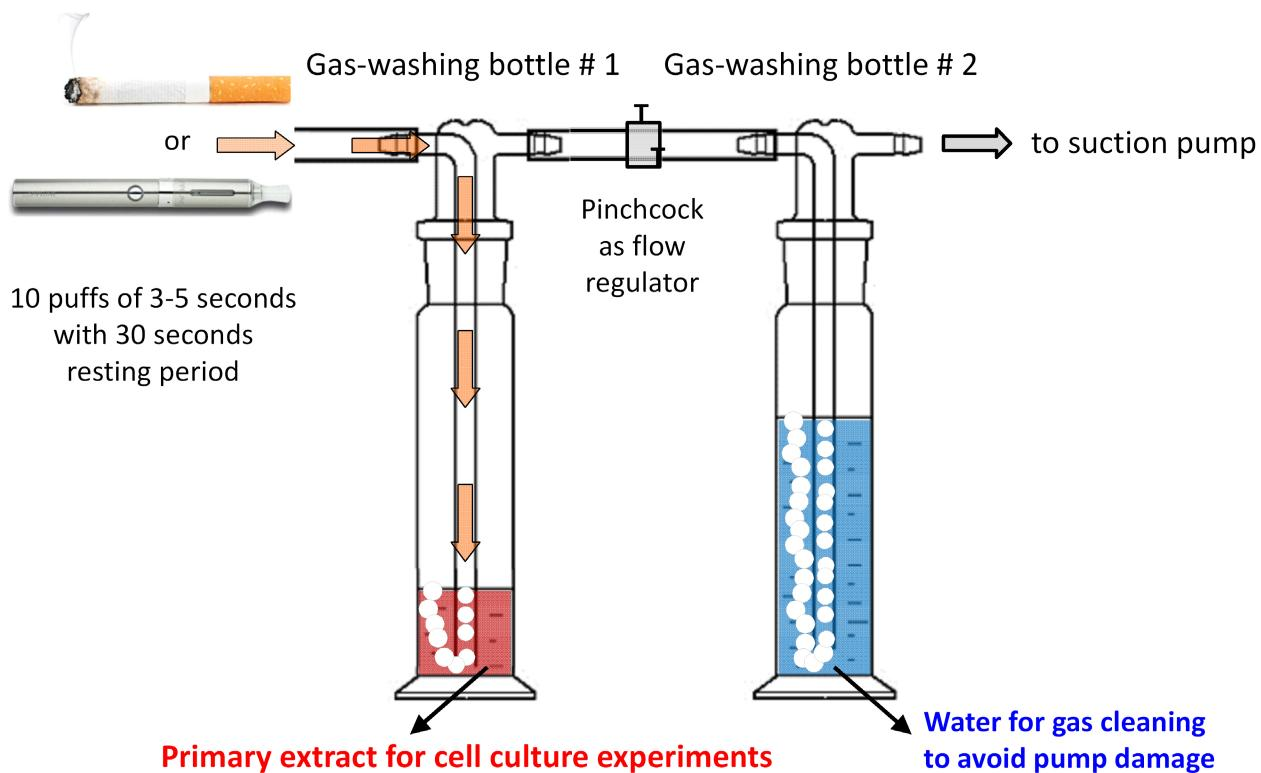
**Figure 1:** Experimental setup for a realistic simulation of cigarette smoking or vaping. The suction pump on the right generates an adjustable underpressure which aspirates the smoke or vapour and passes it into the culture medium in the left gas-washing bottle # 1. This yields the primary extract which is used for the further experiments.
