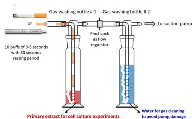
**Fig. 1:** Experimental setup for simulation of cigarette smoking or vaping. The suction pump on the right generates an adjustable underpressure which aspirates the smoke or vapour and bubbles it into the culture medium in the left gas-washing bottle # 1. This yields the primary extract.
