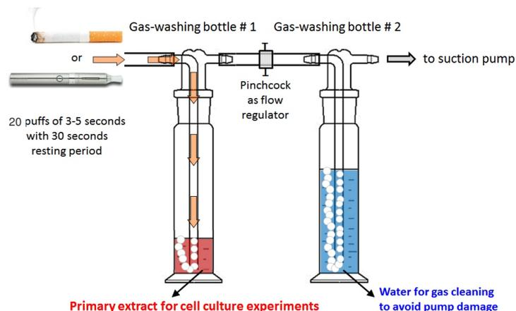
**Figure 1:** Experimental setup for simulation of cigarette smoking or vaping. The suction pump on the right generates an adjustable underpressure which aspirates the smoke or vapour and bubbles it into the culture medium in the left gas-washing bottle # 1. This yields the primary extract.
