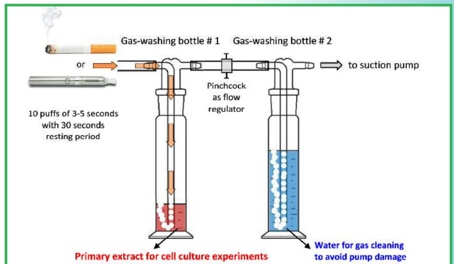
Figure 1: Experimental setup for a realistic simulation of cigarette smoking or vaping. The suction pump on the right generates an adjustable underpressure which aspirates the smoke or vapour and bubbles it into the culture medium in the left gas-washing bottle # 1. This yields the primary extract which is used either undiluted or diluted for the further cell culture experiments. The right gas-washing bottle # 2 is only for gas cleaning to avoid pump damage.
